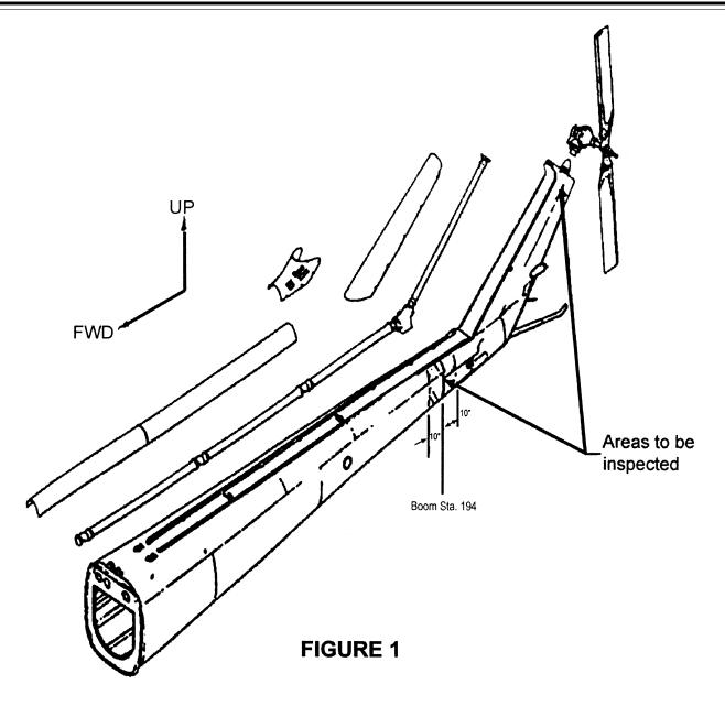
Note 2: The tailboom skin joint at BS 194 is located at the bulkhead just forward of the attachment area for the 42-degree tail rotor gearbox assembly (42-degree gearbox) and the intersection between the vertical fin forward canted bulkhead and the lower tailboom skin.
