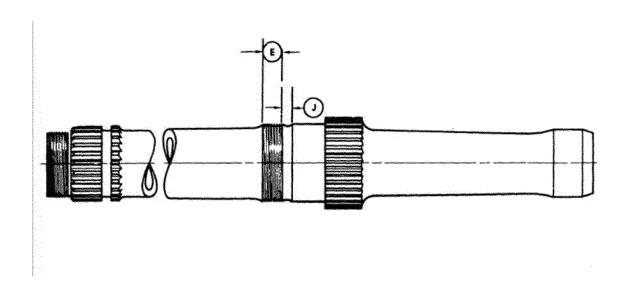
(2) If there is a crack, pitting, or corrosion, before further flight, replace the mast with an airworthy mast.
