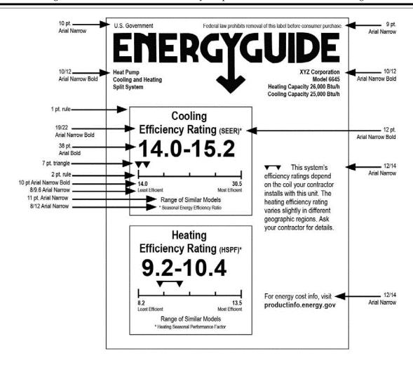
Prototype Label 4 – Split-system Heat Pump (only for units manufactured on or after the compliance date of DOE regional efficiency standards in 10 CFR part 430)
