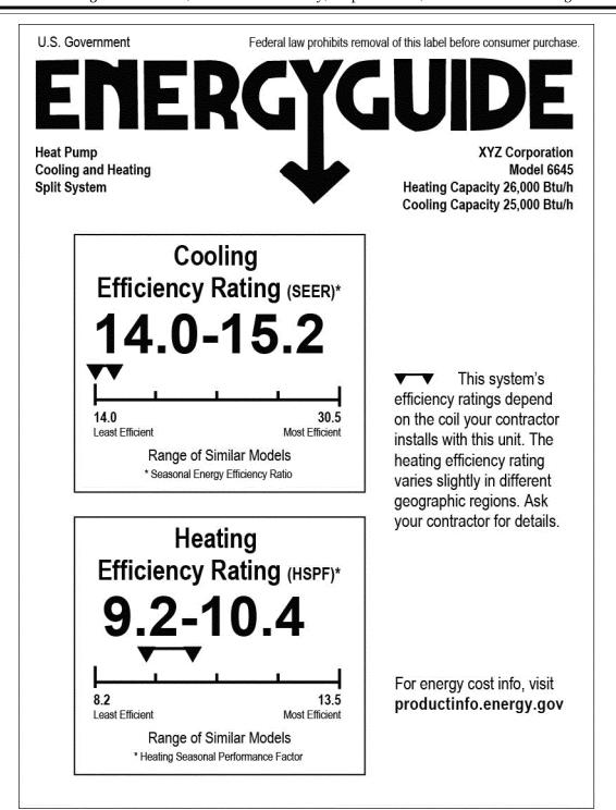
Sample Label 8 – Split-system Heat Pump (only for units manufactured on or after the compliance date of DOE regional efficiency standards in 10 CFR part 430)
