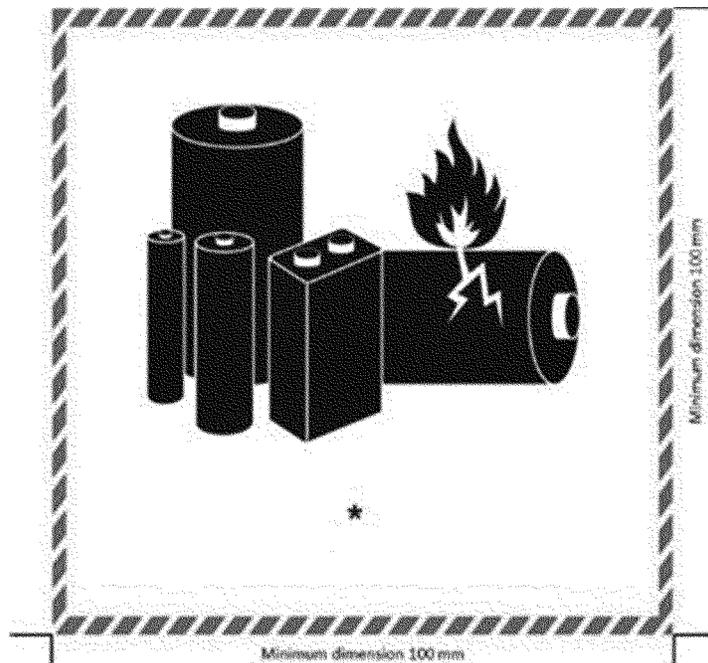
(A) The mark must be in the form of a rectangle or a square with hatched edging. The mark must be not less than 100 mm (3.9 inches) wide by 100 mm (3.9 inches) high, and the minimum width of the hatching must be 5 mm (0.2 inches), except marks of 100 mm (3.9 inches) wide by 70 mm (2.8 inches) high
