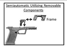
(v) AR-15-type, and Beretta AR-70-type firearms: the lower part of the weapon that provides housing for the trigger mechanism and hammer.
