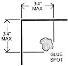
g. Continuous glue lines may be used as cover-to-cover seals and must be placed along the entire length of the open edge and end no more than <sup>3</sup>/<sub>4</sub>-inch from the open ends (see Exhibit 201.3.11.g).
