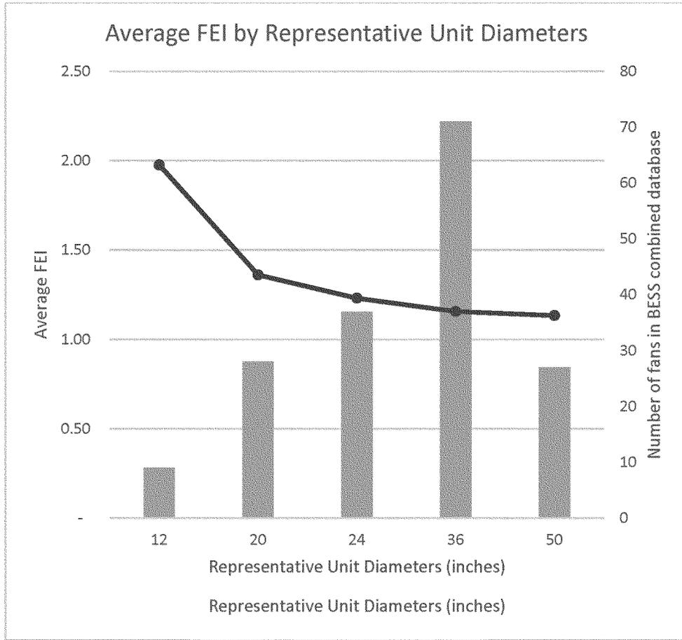
**Figure 1: Average FEI and Number of Fans in the BESS Combined Database as a Function of Representative Diameter.**
