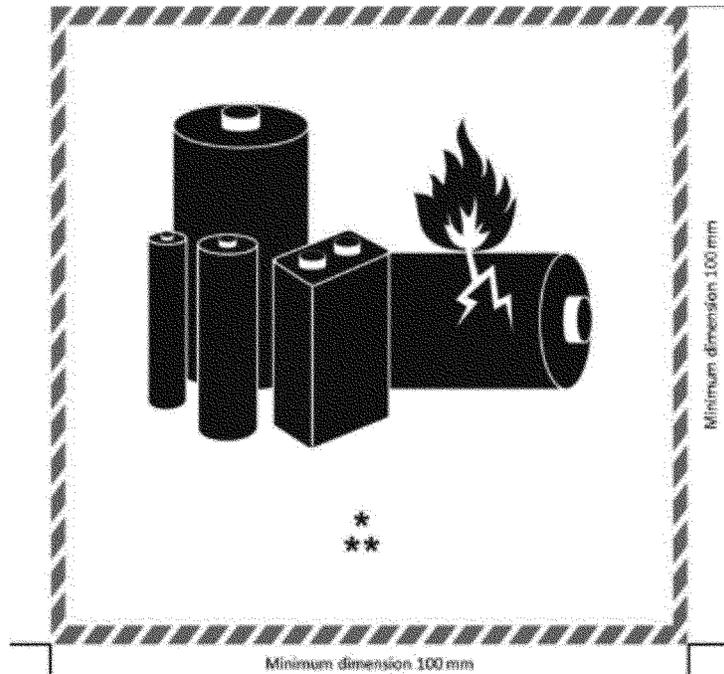
(A) The mark must be in the form of a rectangle or a square with hatched edging. The mark must be not less than 100 mm (3.9 inches) wide by 100 mm (3.9 inches) high and the minimum width of the hatching must be 5 mm (0.2 inches), except marks of 100 mm (3.9 inches) wide by 70 mm (2.8 inches) high may be used on a package containing lithium batteries when the package is too small for the larger mark;
