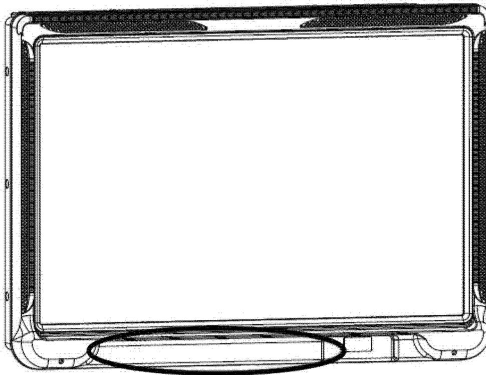
Figure 1 to paragraph (g)(1)(iii); placard location on bezel
