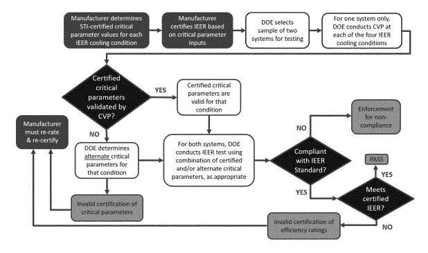
Figure 1: Proposed Process for Conducting the CVP and IEER Testing for DOE Assessment and Enforcement Testing of VRF Multi-split Systems
