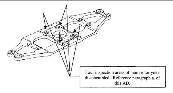
Figure 3. Main Rotor Yoke Inspection Areas
