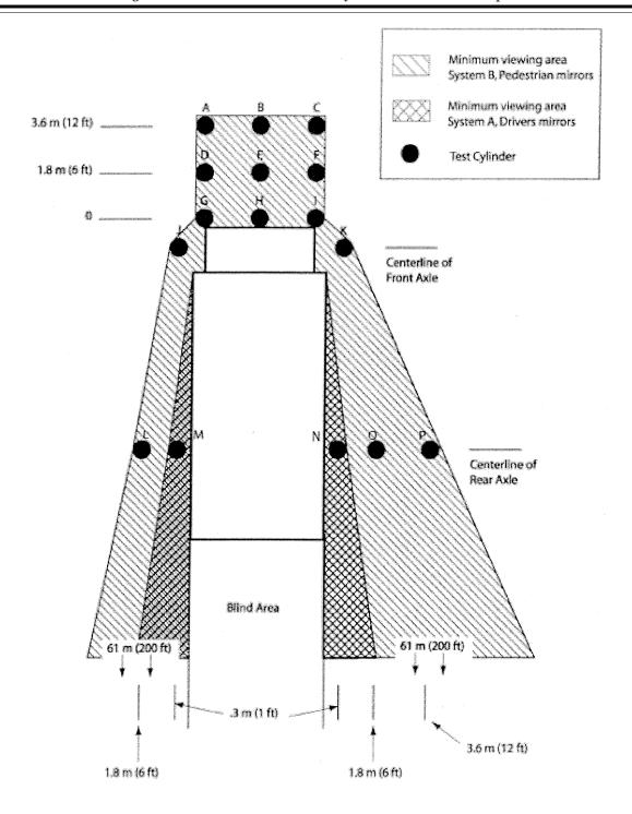
Figure 2, Minimum viewing area, School Bus System A and B Field-Of-View
