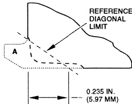
No Area 'A' material remaining and 0.235 inch (5.97 mm) diagonal limit is exceeded.
