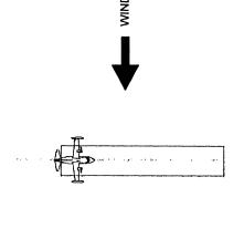
LOWERED AND SMOOTHLY MODULATED. OPPOSITE AIRCRAFT SHOULD NOT BE ALLOWED TO DEVELOP CONTINUES DOWN RUNWAY CENTERLINE. THE PRIOR TO TOUCHDOWN, THE UPWIND WING IS RUDDER IS APPLIED SO THAT AIRCRAFT PATH ANY TENDENCY TO DRIFT DOWNWIND
