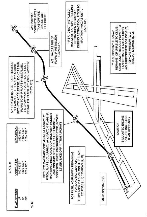
MU-2B J (-35), K (-25), L (-36), M (-26) TAKE-OFF ENGINE FAILURE ON RUNWAY
