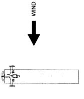
PRIOR TO TOUCHDOWN, THE UPWIND WING IS LOWERED AND SMOOTHLY MODULATED. OPPOSITE RUDDER IS APPLIED SO THAT AIRCRAFT PATH CONTINUES DOWN RUNWAY CENTERLINE. THE AIRCRAFT SHOULD NOT BE ALLOWED TO DEVELOP ANY TENDENCY TO DRIFT DOWNWIND.
