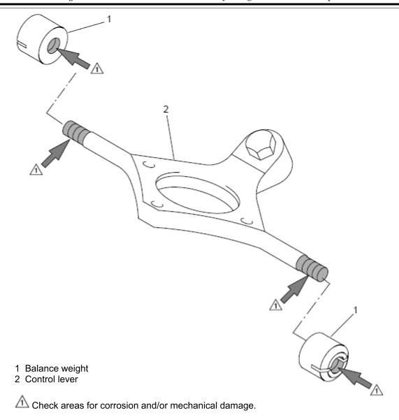
Figure 2 to paragraph (d) Inspection of Balance Weights and Control Lever
