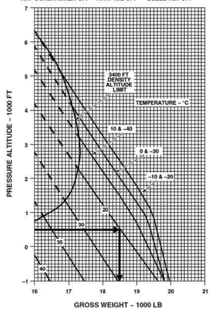
NOTE 1: THIS CHART DEPICTS THE GROSS WEIGHT, PRESSURE ALTITUDE, TEMPERATURE COMBINATION WHERE OEI HOGE CAPABILITY EXISTS USING 30 SECOND OEI POWER WITH A 60 SHP MARGIN.
