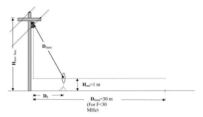
D<sub>slant</sub> is the slant-range distance, in meters; D<sub>h</sub> is the horizontal (lateral) distance between the center of the measurement antenna and the vertical projection of the overhead power line carrying the BPL signals down to the height of the measurement antenna, in meters;
