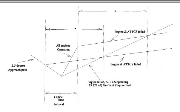
\* The engine and ATTCS failed time interval must be no shorter than the time interval from the point of simultaneous engine and ATTCS failure to a height of 400 feet used to comply with I25.2(b) for ATTCS use during takeoff.
