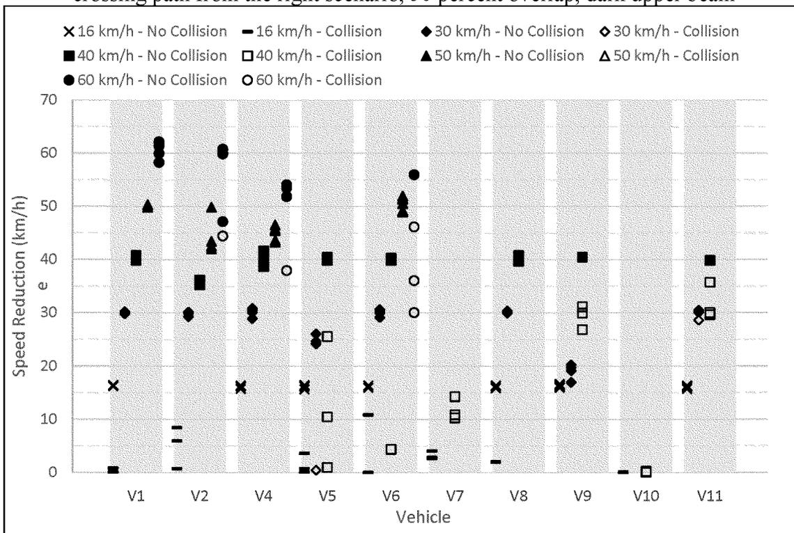
When testing the crossing path scenario from the right with 50 percent overlap at night using the lower beam headlamps, performance was generally worse than when testing with the upper beam headlamps or during the daylight condition. Only two vehicles were
