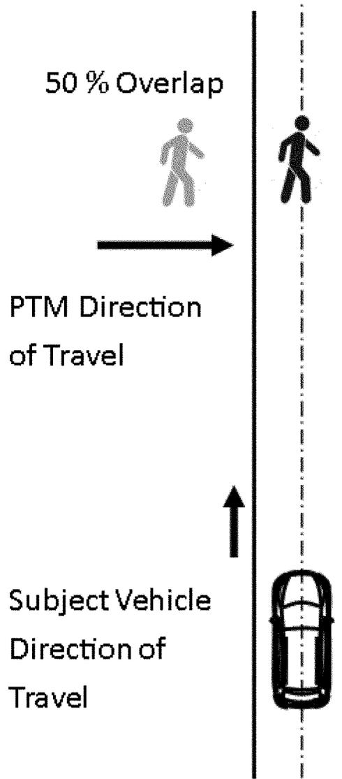
Figure 5 to § 571.127—Setup for Pedestrian, Obstructed
