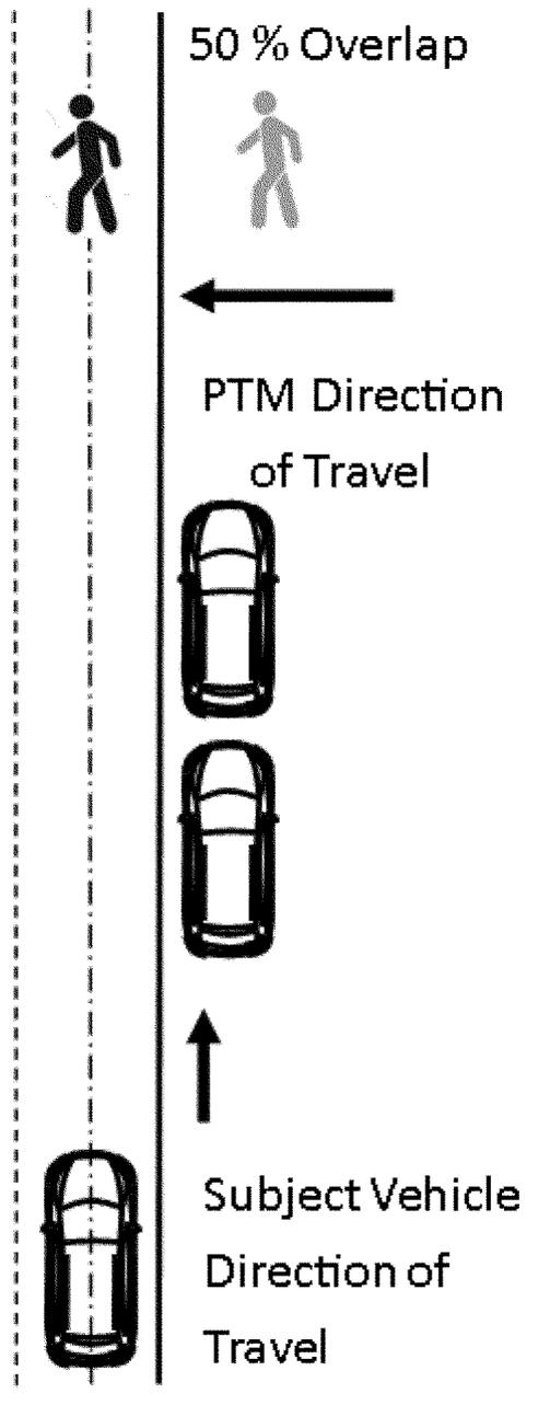
Figure 6 to § 571.127—Setup for Pedestrian Along-Path Stationary
