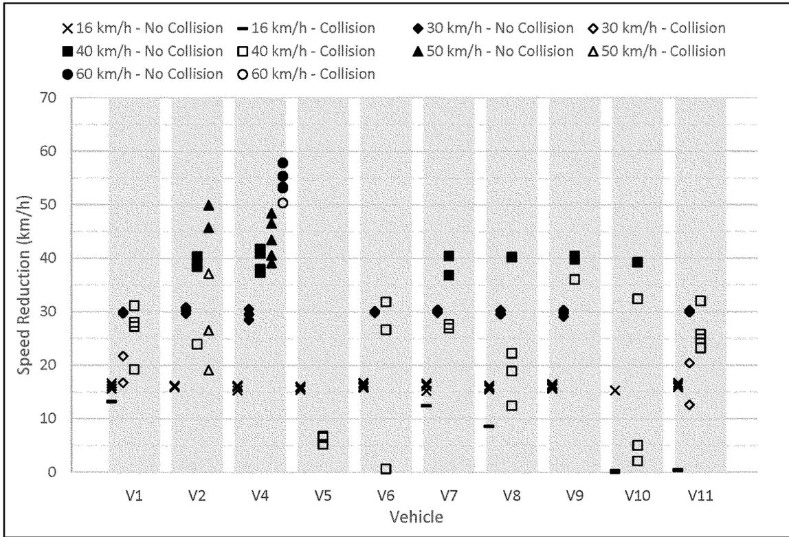
NHTSA’s testing of the running adult pedestrian scenario (pedestrian surrogate travelling at 8 km/h (5 mph)) from the left was performed at speeds from 40 km/h (25 mph) to 60 km/h (37 mph) with a 50 percent overlap during
