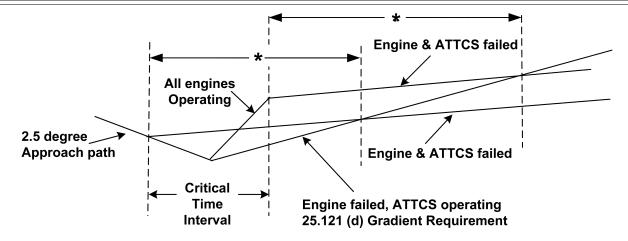
\* The engine and ATTCS failed time interval must be no shorter than the time interval from the point of simultaneous engine and ATTCS failure to a height of 400 feet used to comply with I25.2(b) for ATTCS use during takeoff.
