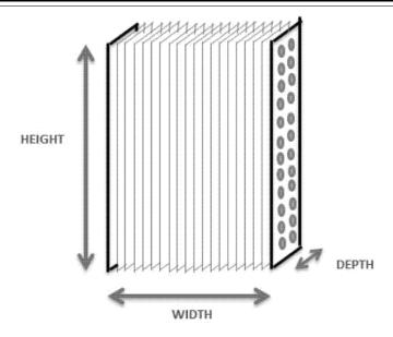
Figure 1: Evaporator Coil Dimensions
