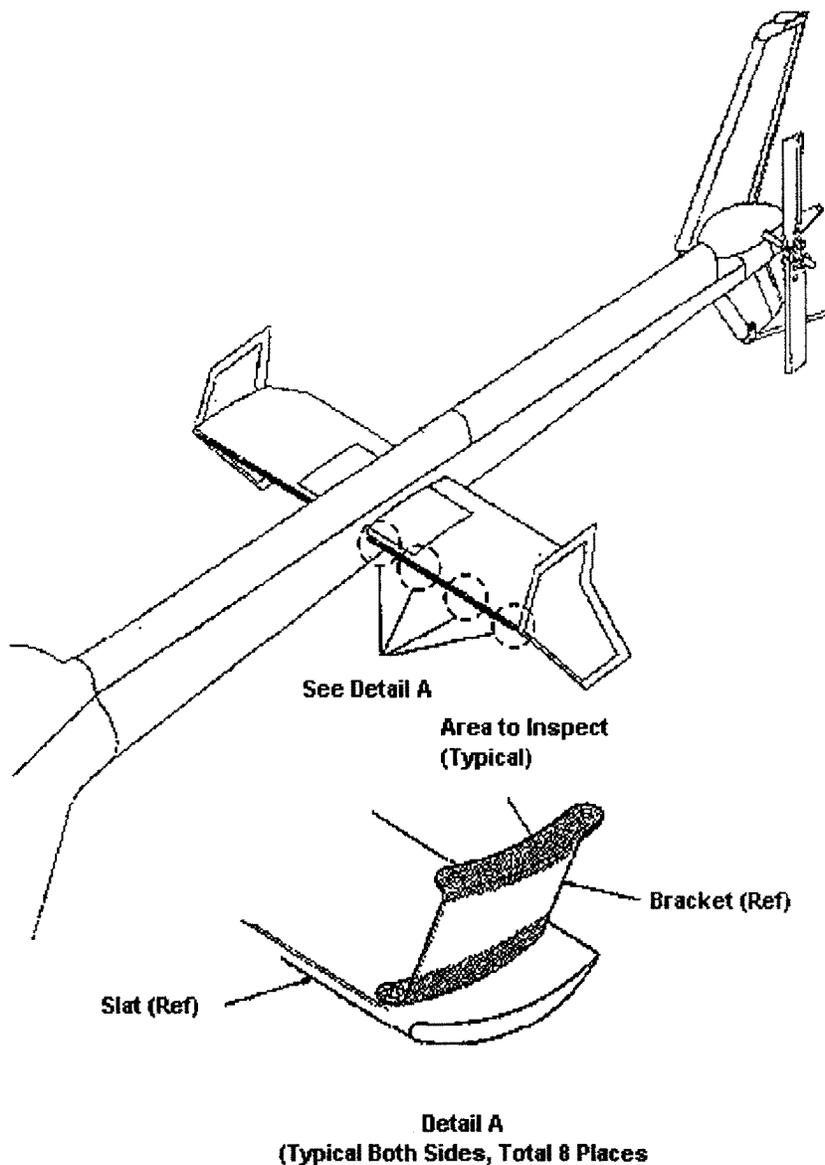
Figure 1. Pre-Flight check of brackets, horizontal stabilizer slats.
