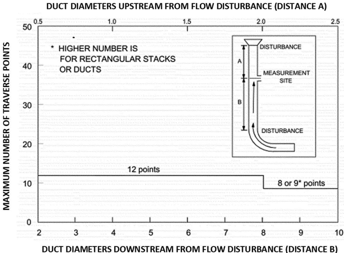
Figure 7. Maximum Number of Required Traverse Points
