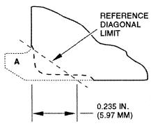
No Area 'A' material remaining and 0.235 inch (5.97 mm) diagonal limit is exceeded.
