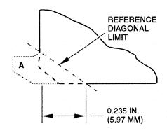
Removal of all Area 'A' material is permitted when axial material removal is less than 0.235 inch (5.97 mm) diagonal limit. Surface shall have a smooth contour and 0.020 inch (0.51 mm) minimum blend radius.
