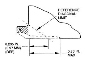
Any remaining Area 'A' lip material is sufficient to permit axial material removal up to 0.38 inch (0.97 mm) limit. Surface shall have a smooth contour and 0.020 inch (0.51 mm) minimum blend radius.
