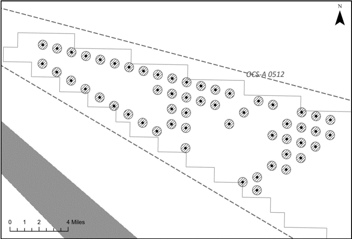
Figure 2 Large scale chartlet showing the positions of the safety zones with a 500-meter safety zone.
