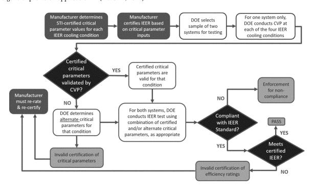
Figure III-1: DOE's Proposed Enforcement Process from the December 2021 VRF TP NOPR
