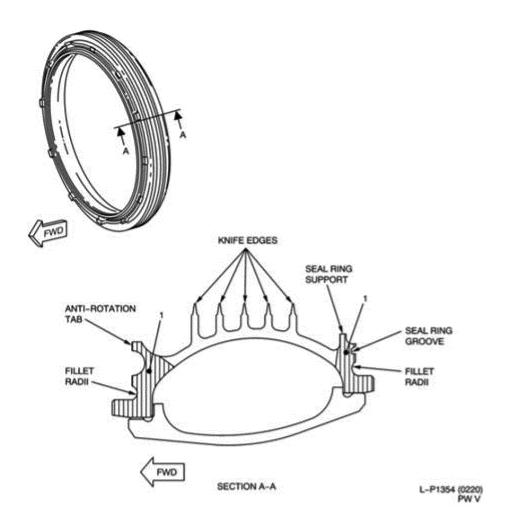
(2) Replacement of HPT 2nd-Stage Air Seal Assembly
