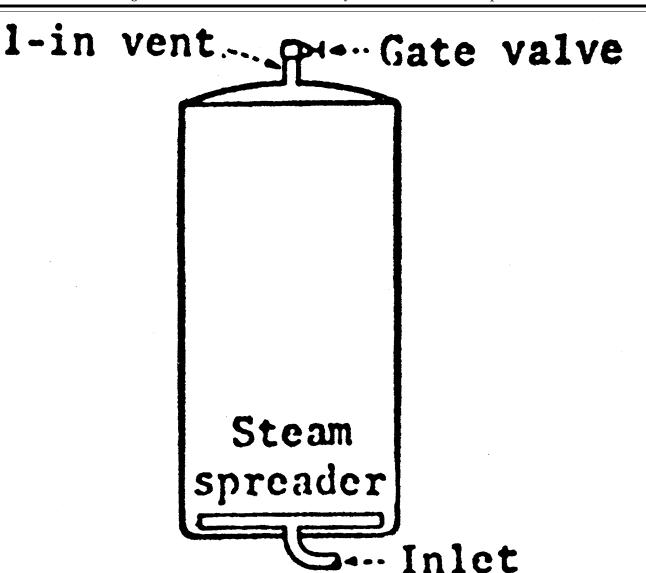
Specifications. A 1-inch (2.5 centimeters) vent in lid or top side, equipped with a 1-inch (2.5 centimeters) gate or plug cock valve and discharging directly into the atmosphere or to a manifold header.
