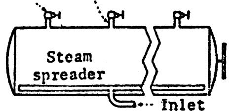
Specifications. One 1-inch (2.5 centimeters) vent for every 5 feet (1.5 meters) of retort length equipped with a gate or plug cock valve and discharging to atmosphere; end vents not more than
