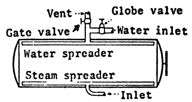
Size of vent and vent valve. For retorts less than 15 feet (4.6 meters) in length, 2 inches (5.1 centimeters); for retorts 15 feet (4.6 meters) and over in length, 2.5 inches (3.8 centimeters).
