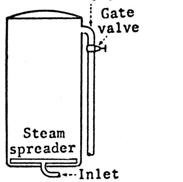
Specifications. A 1.5-inch (3.8 centimeters) overflow pipe equipped with a 1.5-inch (3.8 centimeters) gate or plug cock valve and with not more than 6 feet (1.8 meters) of 1.5-inch (3.8
