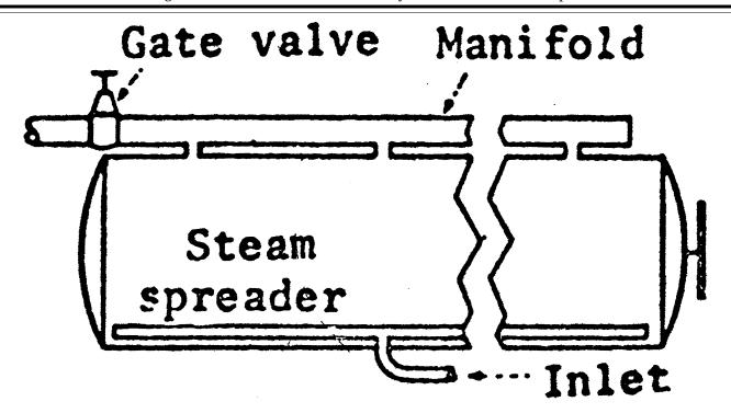
Specifications. One 1-inch (2.5 centimeters) vent for every 5 feet (1.5 meters) of retort length; and vents not over 2.5 feet (76 centimeters) from ends of retort: Size of manifold—for retorts less than 15 feet (4.6 meters) in length,
