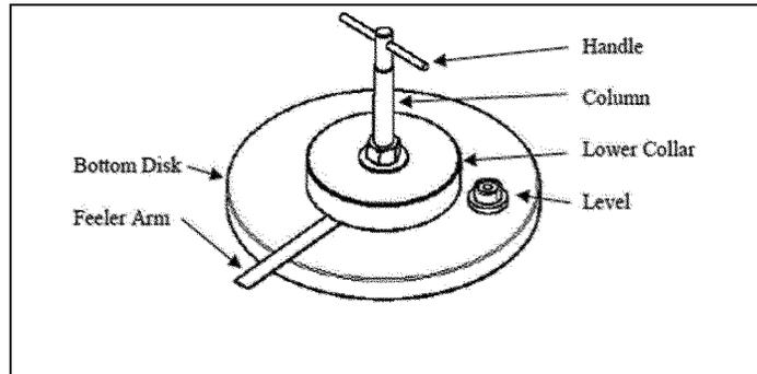
**Figure 10. Mattress Firmness Test Fixture.**
