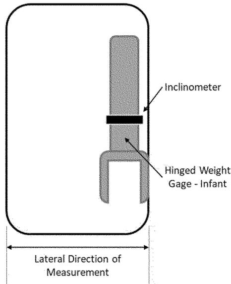
(vii) 7.15.1.5 Remove the Hinged Weight Gauge—Infant (figure 3 to paragraph (b)(25)(iv) of this section). Remove, agitate and replace the mattress (if applicable) to normalize the occupant sleep surface.
