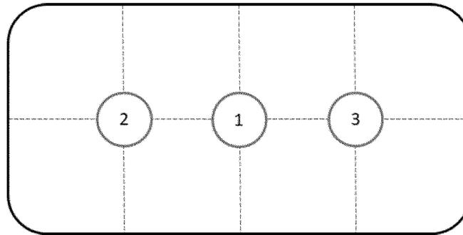
(xiv) 7.13.2.7 Position the test fixture on each of the test locations, with the footprint of the fixture centered on the location, with the bar extending over the centerline and always pointing at the same end of the mattress sleep surface.
